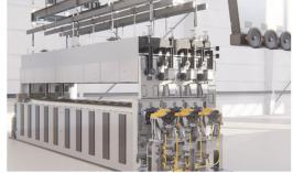
When the glass is lifted out of the tin bath: the dross box. Improved glass quality through a more homogeneous distribution of temperature across the entire width of the glass.
