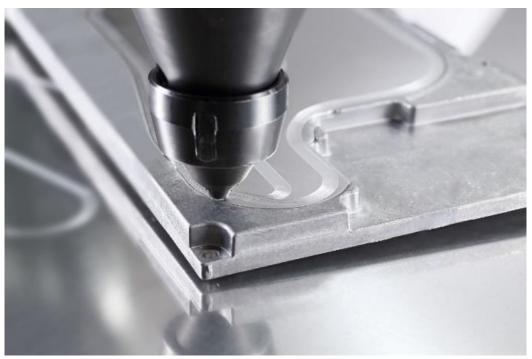
In friction stir welding, the workpieces are joined using friction, pressure and heat. This results in a durable, media and pressure-tight weld seam.
