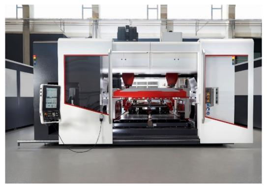
The double-spindle FSW gantry machine D-DSM from Grenzebach enables even faster and more efficient work using its two independently operating welding heads.
