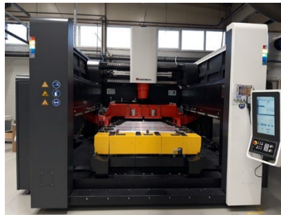
The FSW gantry machine from Grenzbach stands for reliable and reproducible weld seam quality. The four-axis gantry system is designed for high axis dynamics and precise weld path guidance. TPV AUTOMOTIVE uses a total of six FSW gantry machines from Grenzbach for the serial production of battery trays for e-vehicles.
