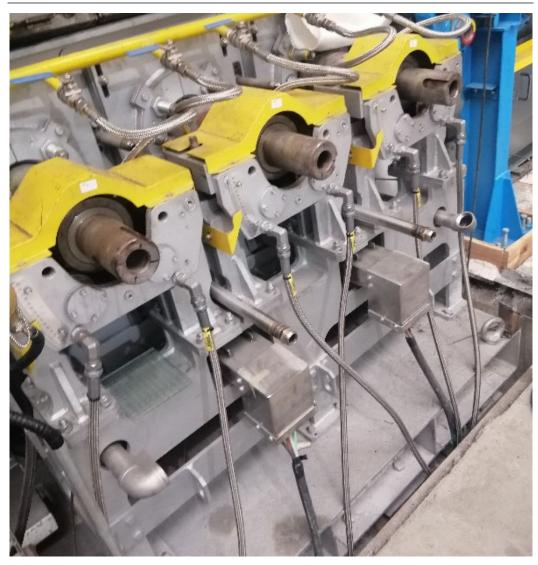
The dross box: Here, for the first time, the pre-strengthened and shaped glass floating on the tin is lifted out by three motorized rollers and transferred to the annealing lehr.
