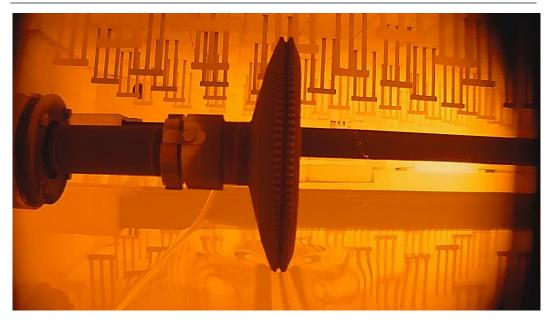
With the top roller machines, the final glass thickness is already set in the tin bath. It is standard at CNUD EFCO GFT for all five degrees of freedom of the top roller to be automated: rotation, parallel stroke, angle of inclination, angle of engagement and depth of entry. The process is controlled remotely from the tin bath control room – no manual intervention at spot is required.
