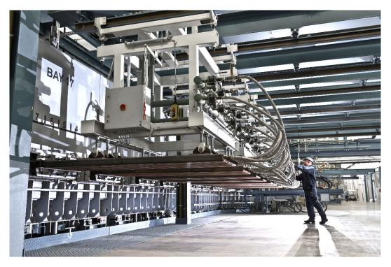
CNUD EFCO GFT supplies the complete tin bath with everything that goes with it. In addition to design and construction, intelligent combination is also crucial for optimum plant operation. All components are manufactured in-house: the tin bath with its highly complex equipment, the top rollers and the dross box.
