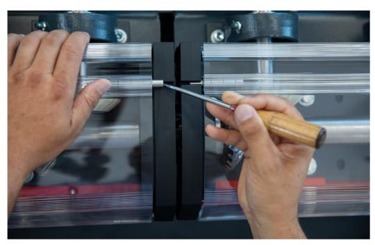
CE-conformal quick release fasteners make the drive train easily accessible. Thanks to the quick lock system, access for maintenance work is now much easier and faster.
