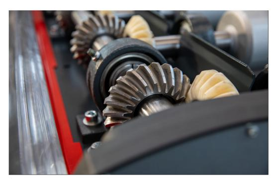
Gentle glass transport along the entire line: Newly developed bevel gears are used for power transmission to the respective support rollers. They not only enable smooth and gentle running, but above all guarantee even more precise positioning.
