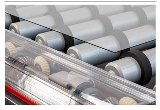
Access to the conveyor system is possible via a continuous transparent protective cover. This means a clear view of the key components at all times.
