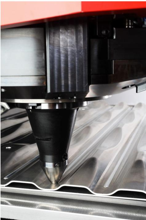
*During friction stir welding, a rotating tool generates the required process heat with friction and pressure at the process point. The heated material turns malleable and is stirred along the seam by the rotation of the tool.*
