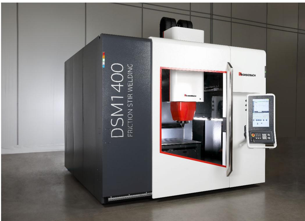
*The compact 4-axis gantry machines of the DSM series (DSM = Dynamic Stirring Machine) stand for high axis dynamics, precise web guidance and intuitive control and operating concept.*
