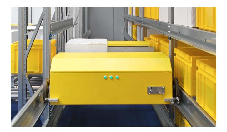
In the world of intralogistics, shuttle systems have already been around for decades, and thus constitute an extremely mature technology. The racks can be installed up to a height of 18 meters. Conveying technology and vertical lifters are required for operation. This infrastructure requires certain structural conditions, meaning that not every facility is suitable for this system, and the corresponding project lead time must be taken into account.
