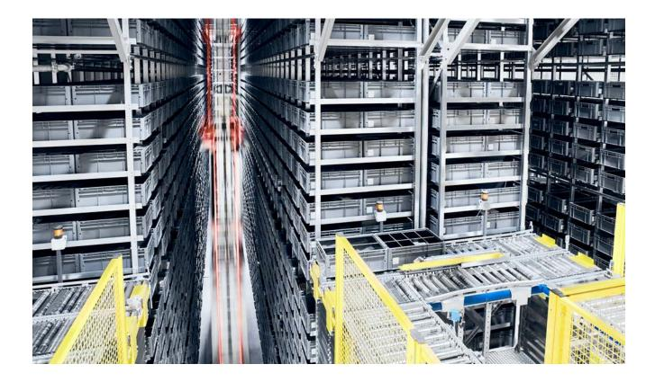
They are one of the absolute classics of intralogistics – automated small-parts warehouses in which goods are stored and retrieved using AS/RS systems. The racks can be up to 22 meters high – given this ceiling height and double-deep racking, it is possible to achieve a high storage density. Automated small-parts warehouses can only be implemented in specially constructed new buildings. The construction of such buildings normally requires a lead time of about 12 to 18 months.
