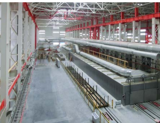
Grenzebach gypsum block dryer, view from the inlet side
