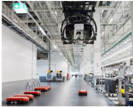
For the manufacturing of the new Audi A8 in Neckarsulm, Grenzebach incorporates a system solution with 30 L1200S Automated Guided Vehicles (AGVs) for high-performance process networking. This L1200S transports up to 1.2 tons lengthwise or crosswise – and can also turn on the spot. Thanks to the very low height, the L1200S can go under most load carrier (tables, trolleys, racks, shelves), lifting it and transporting it to the specified destination.
