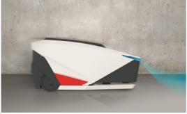
The further developed tugger is able to automatically couple and uncouple trolleys - and a multitude of different trailer couplings allow a flexible and repetitive automatic transport of goods on the inner-company ways. In the curves, the new model now performs a turning radius of 1.2 m, which means that the available motion space at the customer's facilities is used in an optimum way.
