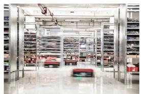
The L600 is used as "goods-to-person-system" in many different ways, here at BLG Logistics. This AGV allows the customer to organize even highly demanding logistics surfaces quickly, economically, multistory and are flexibly scalable. The compact vehicle "L600" from Grenzebach moves beneath goods carriers, lifts them and transports them towards the picking place.
