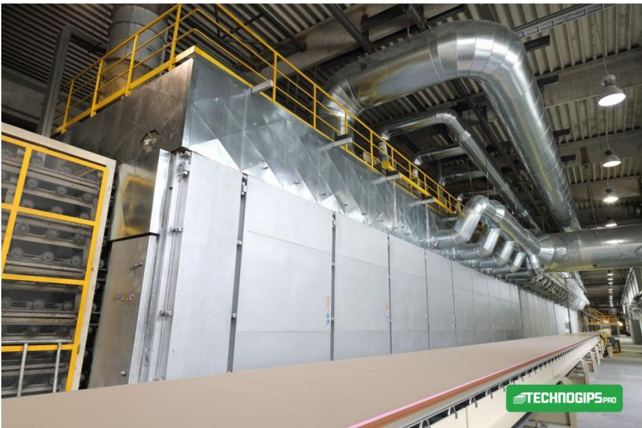
*Upgrading made easy: The cross-flow jet dryer has a modular design, allowing further sections to be added - and thus the capacity to be increased - in an easy way.*
