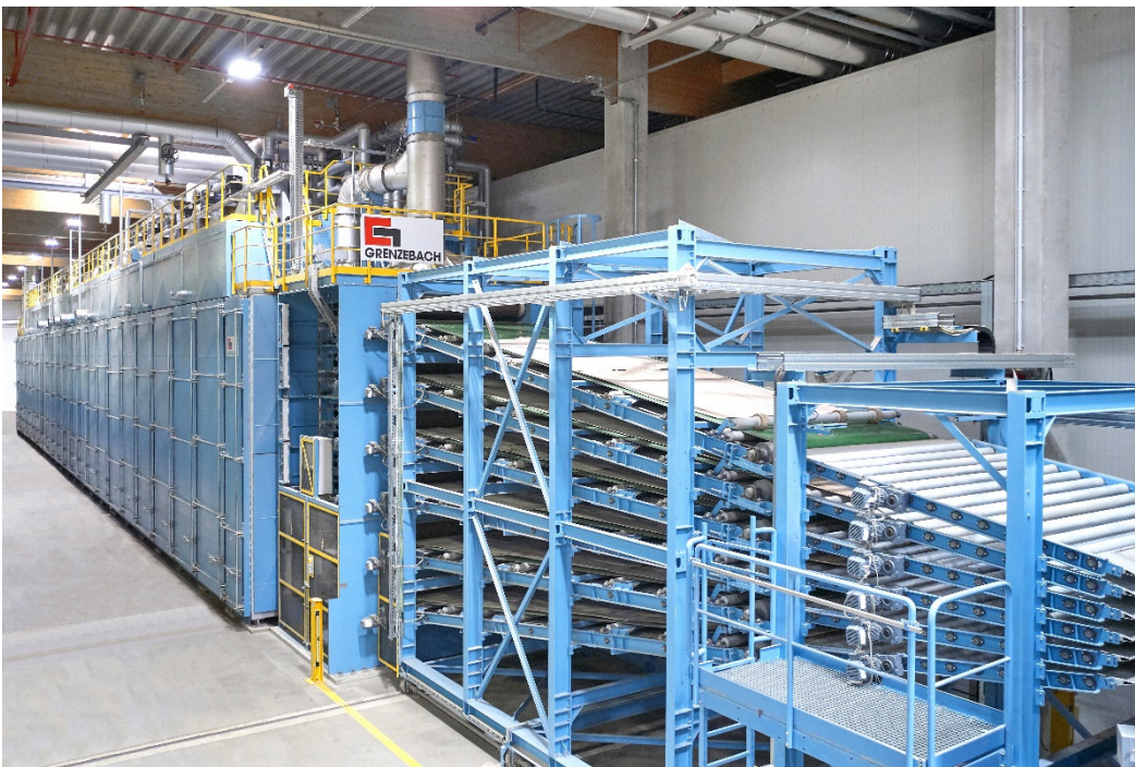
Reliable feeding of the veneers, which have a fibre length of 2,100 mm and a fibre width of 2,200 mm, in the feeder area, trouble-free veneer transport through and smooth and proper discharge from the dryer.
