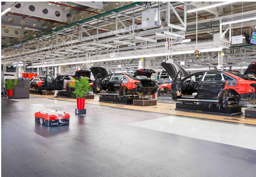
The AGVs use contour navigation in the workshop to reach their destination. Certified laser scanners on the vehicle calculate the vehicle's position by reflection of environment characteristics. Contact loops or other optical means on the shop floor are not necessary. Source: Grenzebach Maschinenbau GmbH
