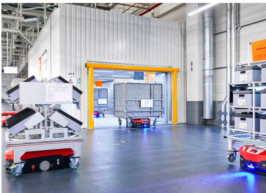
*The routes between the supply and the work stations occur on three levels - the AGVs are mobile via elevators on the ground floor, the upper and the lower floor.*
