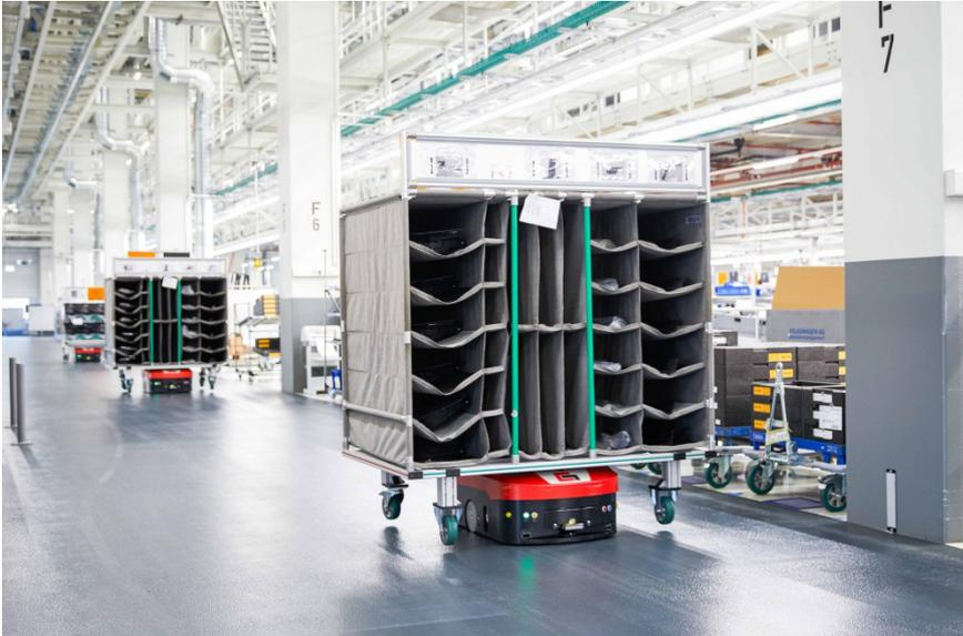
*Sequence vehicles filled with components are transported automatically and intrinsically safe with the L1200S, moving beneath it, from the supply stations to the work station they are requested at - this is ensured by the laser scanner.*
