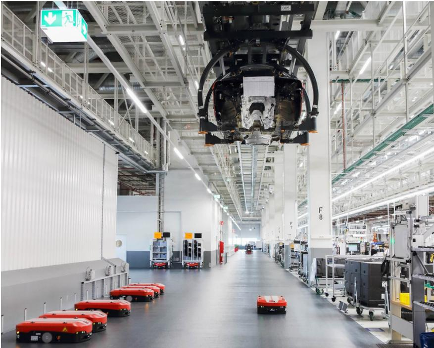
The manufacturing of the new Audi A8 in Neckarsulm follows the principles of the smart factory. The core piece for the intelligent process network consists of 30 Automated Guided Vehicles (AGVs), type L1200S. They are integrated into the smart factory using the Fleet Manager and their main task is the timely supply of custom-fit components to the manufacturing islands. Source: Grenzebach Maschinenbau GmbH
