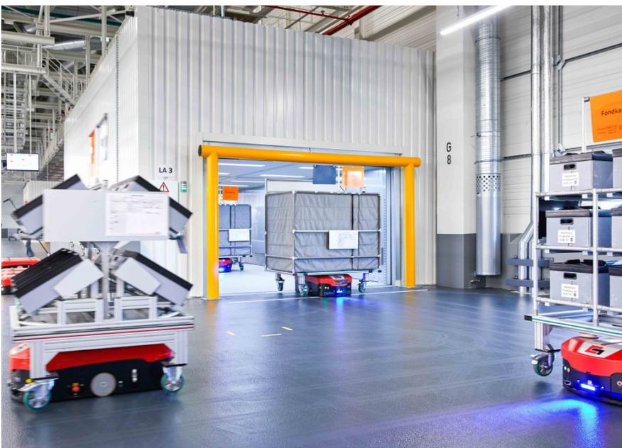
*The routes between the supply and the work stations occur on three levels - the AGVs are mobile via elevators on the ground floor, the upper and the lower floor.*
