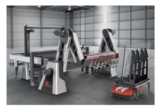
Combined with the accumulator, conveyor line and Automated Guided Vehicles (AGV), the Tin-Air-Speed-Stacker shows numerous advantages. With the new double-arm kinematics connected to an ideal matching infeed section with glass sheet accumulator, a highly efficient, fast and flexible stacking cell for small glass sizes up to 2m was created.
