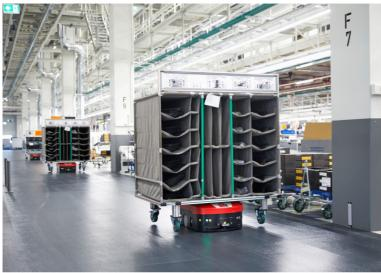
This Automatic Guided Vehicle (AGV) of Grenzebach, the L1200S, transports up to 1.2 tons lengthwise or crosswise – and can also turn on the spot. Thanks to the very low height, the L1200S can go under most load carrier (tables, trolleys, racks, shelves), lifting it and transporting it to the specified
