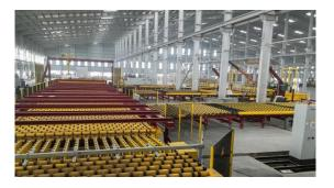
From the main line three sidelines lead towards stackers and rotary platforms and Jumbo stacker at the line end.
