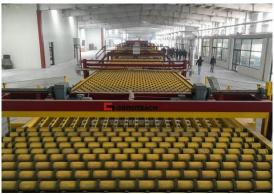
With a length of approx. 190 m, the Cold End equipment from Grenzebach is the end of the new float glass production line from Gold Glass. The picture shows the main line course towards the continuous ribbon area.
