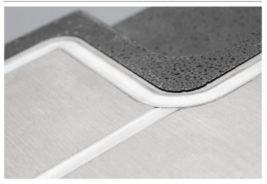
Optimum joints: Lost foam cast with uneven surface can be processed optimally with the friction stir welding technology.
