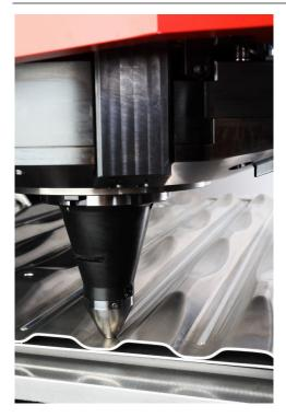
During friction stir welding, a rotating tool generates the required process heat with friction and pressure at the process point. The heated material turns malleable and is stirred along the seam by the rotation of the tool.
