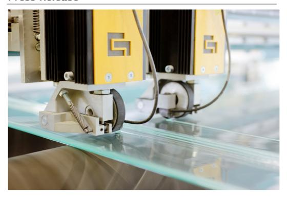
Here, the cutting technology is shown, working on the basis of the previous camera system. On the left side, you can see the gross cutting tool and on the right side the cutting tool for the net cut. The distance between the net cut tool and the knurl mark seems to be comparatively quite big. By means of the Float Scan Edge-digital, users can completely use this optimization potential: By means of the cutting tool, they get very close to the top roller trace and the net glass ribbon gets wider.
