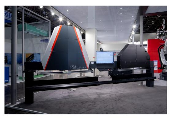
International premiere in Düsseldorf: At the glasstec the new FSE-d (Float Scan Edge-digital) was presented for the first time. On the left side in the picture, you see the new version of the camera system, by means of which the position of the top roller trace can now be determined even more exactly and reliably. This leads to more square meters in glass and the yield rises.
