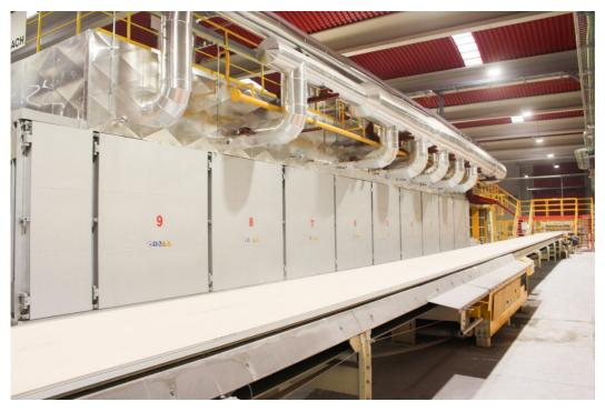
Focus on the dryer: The intelligent dryer control system provides for maximum energy efficiency and keeps emissions at low levels.
