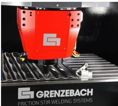
The deciding factor for the weld seam and surface quality is the control of the process parameters, primarily the contact pressure. With the sensor system of the welding head, the contact pressure is reported back to the machine and process control and together with the individual axis of the lead machine represents the force control circuit.
