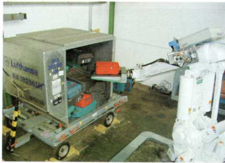
■ The automatic baggage handling system from Grenzebach employs a robotic arm to grab items from the conveyor belt and transfer them into a unit load device.
