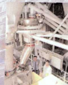
Fully automatic dosing, weighing and mixing of aggregates, binder materials, fibres and pigments
