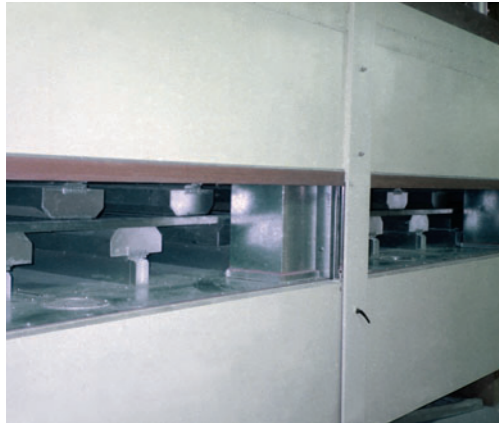
Air flotation dryer with opened door
